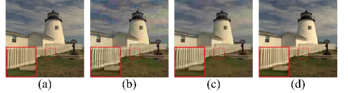
Fig. 10 The visual comparison deblocking results of image LightHouse3 on the LIVE1 (image size: 256 \times 256 ) dataset at Q = 10 . (a) Original image. (b) JPEG compressed image (PSNR = 27.52 dB, SSIM = 0.7561). (c) SA-DCT (PSNR = 28.33 dB, SSIM = 0.7786). (d) Ours (PSNR = 28.78 dB, SSIM = 0.7951).
