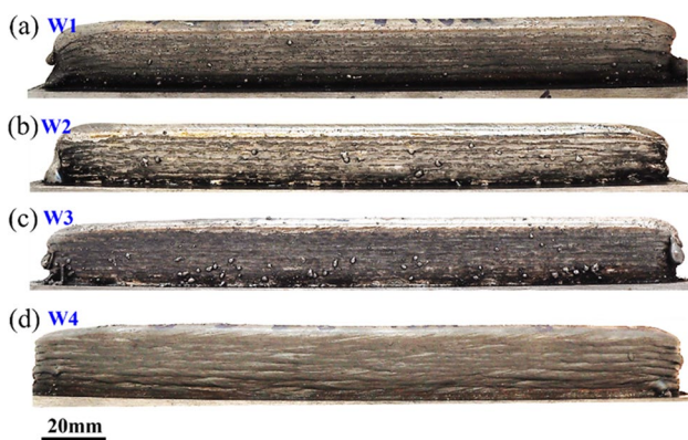
Fig. 4 Side surface morphology of single-pass 300 M wall processes under different local shielding gas mixtures: a 97.5% Ar+2.5% CO 2 , b 92% Ar+8% CO 2 , c 80% Ar+20% CO 2 , and d 60% Ar+38% He+2% CO 2
