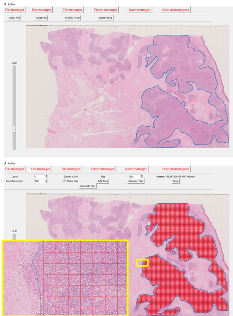
Figure 4. Representative screenshots of TilerPath during the datasets creation. Each whole slide image may be opened and explored at the original magnification provided by the scanner. A File manager tool allows the user to select the path in which are stored the scanned slides, and to select a specific output path in which the tiles generated will be stored. The ROI manager tool allows the user to outline the tissue area that will be tiled. Tiles dimension and capture magnification may be managed within the Tiles manager tool, tiles don't overlap each other and remain confined within the selected area (yellow box). Filters manager tool allow the user to run algorithms for the tiles quality control, with this tool cellularity cut-off may be selected and tiles with tissue artifacts automatically excluded from the export. To use Filters manager tool a Graphical Processing Unit (GPU) is recommended, users without GPU can skip Filters manager without interfering with the other functions of the system. Finally, the Save manager tool allows to export the generated tiles to specific directory created by the user. TilerPath was specifically designed to run on Windows 10 or further version.
