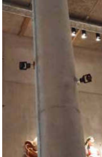
On left and right: prisms in the ship (left) and around it (right) used to mark the position of the TS.
