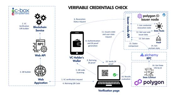
Figure 9. Verification of verifiable credentials in C-Box<sup>®</sup>.
