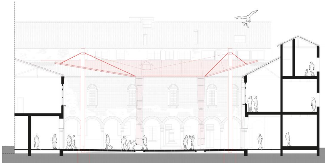
Figure 3: Section of the courtyard with the hypothesized roof
