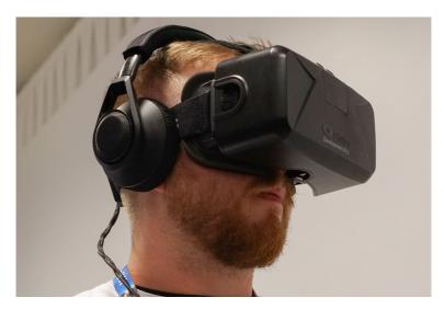
Figure 3: Head-mounted display, Oculus Rift.
