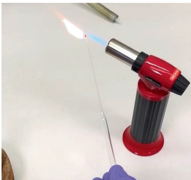
Figure 15. A terpene oligomeric residue burning vigorously in air after being lit with an open flame.
