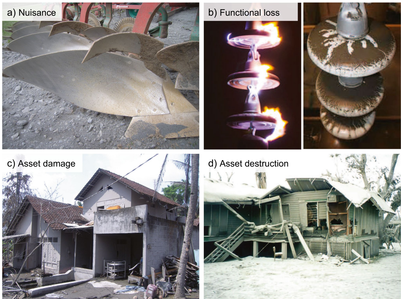
Fig. 3 Photos of impacts to the built environment at different consequence severity and for different volcanic hazards: (a) Nuisance: minor corrosion to farming equipment that occurred overnight (observed by the photographer and confirmed by the farmer) as a result of gas and/or tephra during the explosive phase of the 2010 eruption of Eyjafjallajökull, Iceland (credit: SF Jenkins); (b) Functionality loss: tephra induced flashover (short-circuiting) across a porcelain insulator during laboratory experiments (left) and the thin layer of damp tephra responsible (right) (credit: JB Wardman and G Wil-
