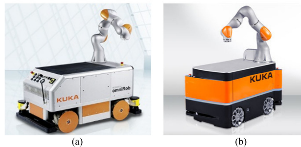
Fig. 1. KUKA mobile manipulators as representative industrial mobile manipulators. (a) KUKA OmniRob, (b) KUKA KMR iiwa.
