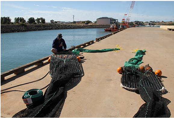
Figure 1. Nordmøre-grids designed to reduce bycatches of cuttlefish in penaeid trawls being assembled on a quayside (photograph by M. Broadhurst).
