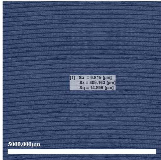
(b) Feed rate = 0.2 mm/rev and rake angle = -6^\circ at MRV = 172 \times 10^5 \text{ mm}^3
