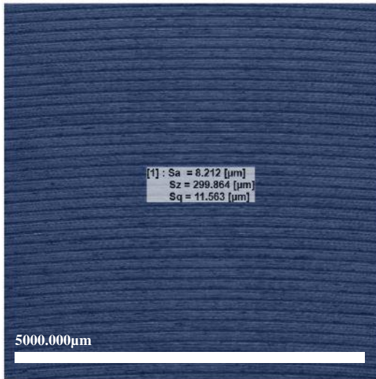
(a) Feed rate = 0.2 mm/rev and rake angle = -6^\circ at MRV = 138 \times 10^5 \text{ mm}^3
