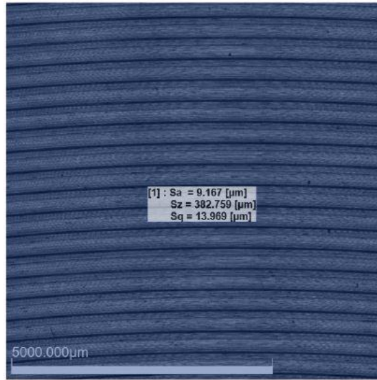
(d) Feed rate = 0.4 mm/rev and rake angle = -9^\circ at MRV = 172 \times 10^5 \text{ mm}^3
