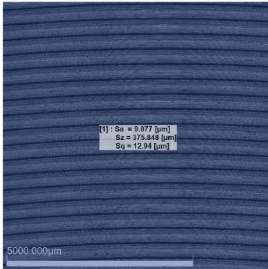
(c) Feed rate = 0.4 mm/rev and rake angle = -9^\circ at MRV = 138 \times 10^5 \text{ mm}^3
