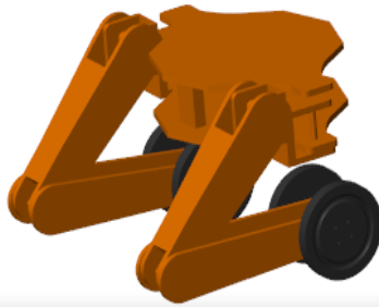
Figure 3.6: The robot design that has been import from Solidworks to MATLAB Simulink.
