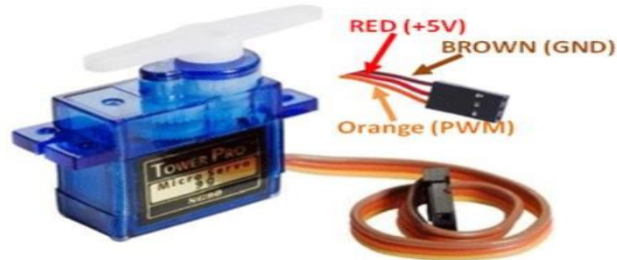
Figure 2.2.1 1 Servomotor and the Connectors
