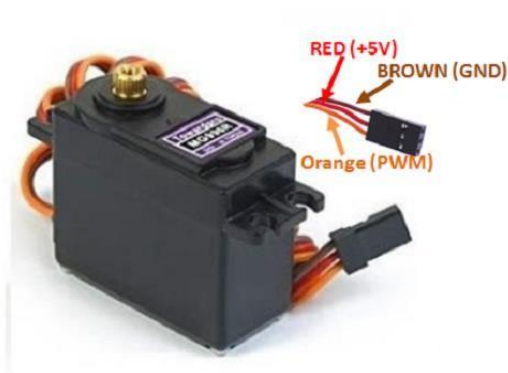
Figure 3.3.1 1 shows the wires of servo motors
