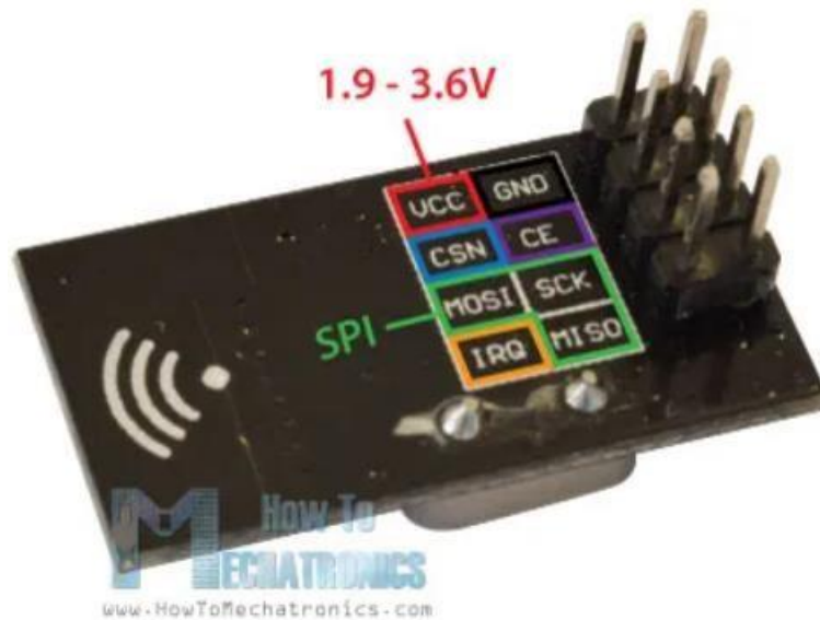
Figure 3.5.2 1 Shows the PINS that need to be connected
