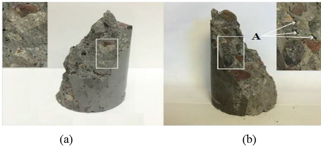
Fig. 12. The ITZ in geopolymer concrete generated from RA (a) and NA (b), where A represents the contemporary interfacial transition zones connecting natural aggregate and geopolymer (Ren and Zhang, 2016).
