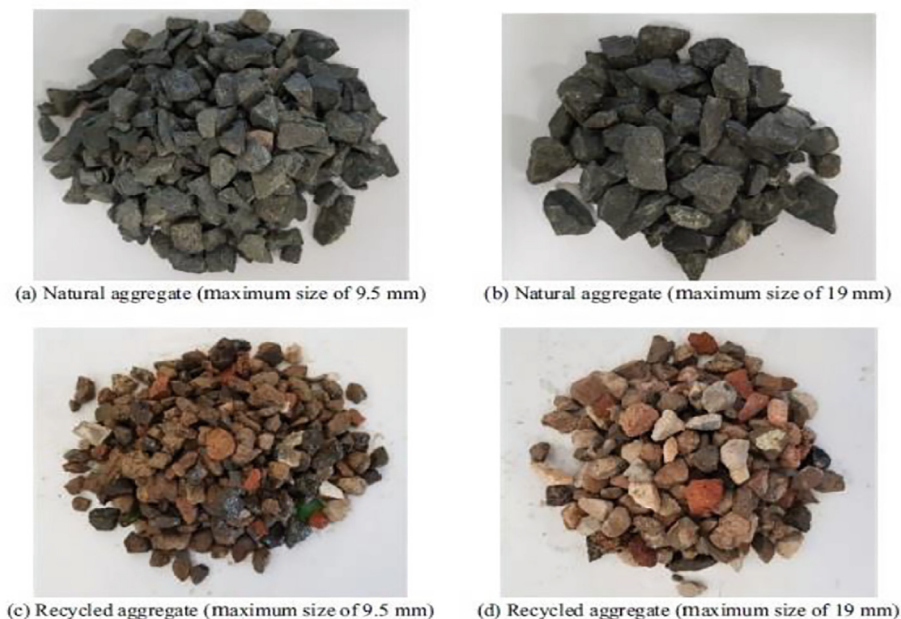
Fig. 3. Comparing the morphology of fine and coarse aggregates used in concrete (Hu et al., 2019).
