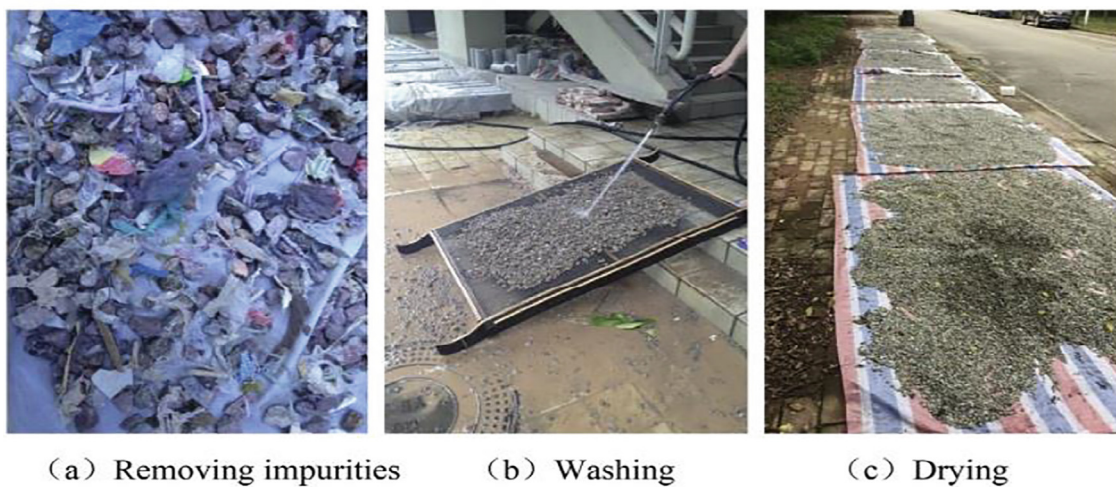
Fig. 1b. The preparation procedure of recycled aggregates (Xie et al., 2019; Xie et al., 2019).
