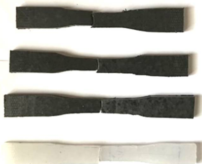
Figure 6. Tensile fractures specimen of LDPE/GO composite.
