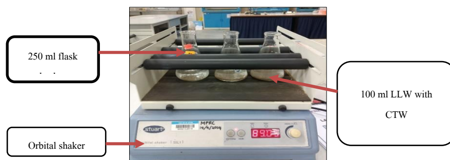
Figure 2. Laundry wastewater during shaking process in a batch method
