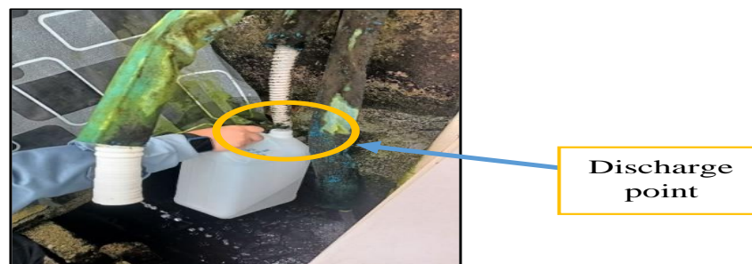
Figure 1. The discharge point of collecting laundry wastewater
