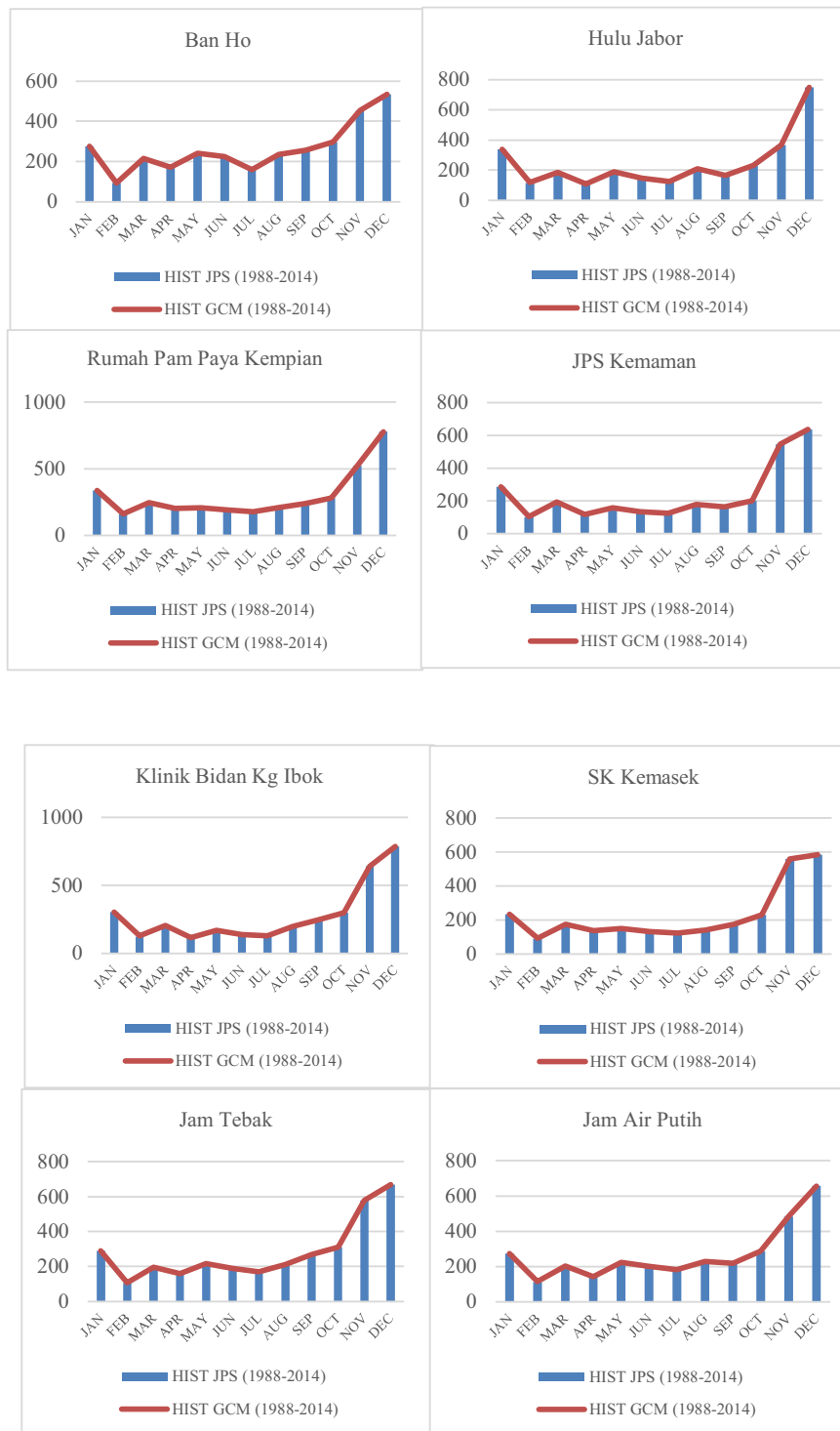
Figure 1. Comparison between historical rainfall data and historical run CMIP6 GCMs model from 1988 until 2014
