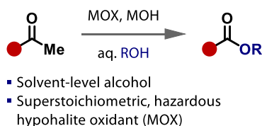
Scheme 1.22. Issues with classical haloform reaction for ester synthesis.
