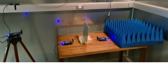
Fig. 4: PlutoSDR based NLOS measurement setup in presence of RF absorbers and interferer.
