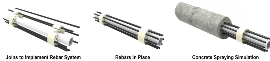
Figure 2. Construction System - PVC Pipes/Rebars/Joins
