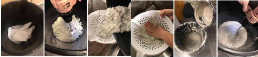
Figure 3. Stoneware slip clay and paper pulp
