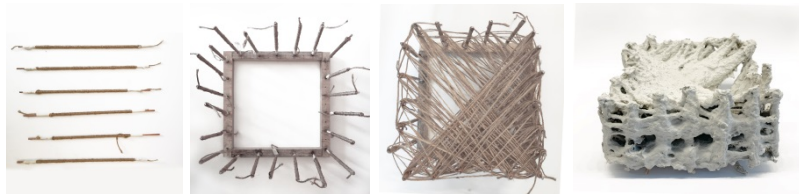
Figure 8. Clay element removal from frame
