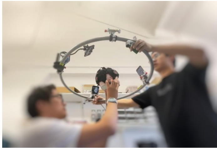
Fig. 4 Photograph of the experimenter holding the phantom and mimicking baby head movement.
