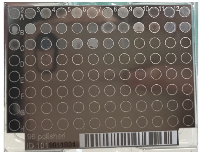
Fig. 2. Photograph of the mass spectrometry plate where samples are plated after either Bruker Sepsityper® or FcMBL-based processing but prior to MALDI-TOF analysis.
