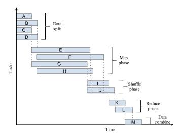
Fig. 6. Execution timeline of the MapReduce tasks depicted in Fig. 5(b)
