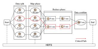
(b) Calculating end-to-end critical path
