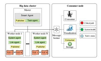
Fig. 3. The high-level implementation of monitoring component
