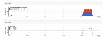
Fig. 6: Sflow tool showing increased traffic on Host1 and Host2 ports during attack
