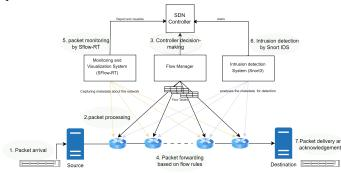
Fig. 3: Proposed Architecture for Intrusion Detection
