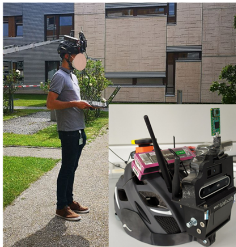
Figure 4. Preliminary setup for data acquisition. 3D printed support located on the helmet
