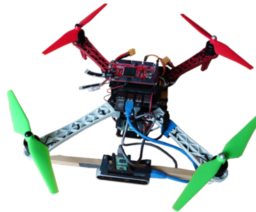
Figure 2. Hardware architecture for indoor flight mounted on DJI-415 Flame Wheel.
