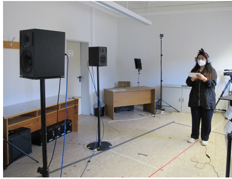
Figure 4.25.: Setup for the listening experiment: Participant wears AKG K1000 headphones with an HTC Vive Tracker attached to it and walks along the translation line marked in red on the floor, switching between test scenes A and B via a graphical user interface provided on a tablet PC.
