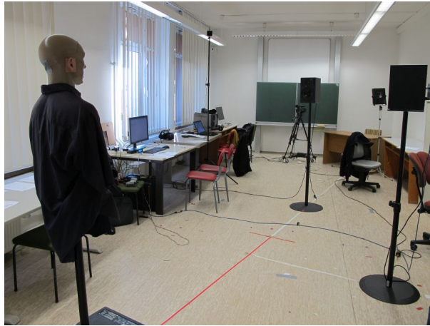
Figure 4.4.: Photos of the BRIR measurement in the seminar room.
