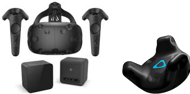
Figure 3.5.: HTC Vive (First generation) with controllers and Lighthouse base stations (1.0) for tracking (picture taken from [235]) and Vive Tracker (2.0).
