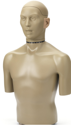
Figure 3.3.: The KEMAR 45BA head-and-torso-simulator from G.R.A.S. Sound & Vibration
