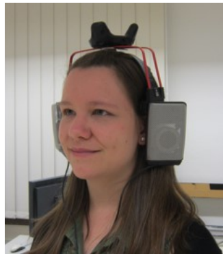
Figure 4.16.: Test person wearing AKG K1000 headphones with a Vive tracker attached to them.
