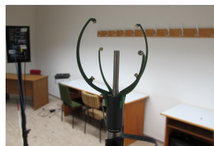
Figure 4.23.: Microphone array to measure directional room impulse responses for analyzing the spatio-temporal pattern of early reflections at the nine listening positions along the translation line.
