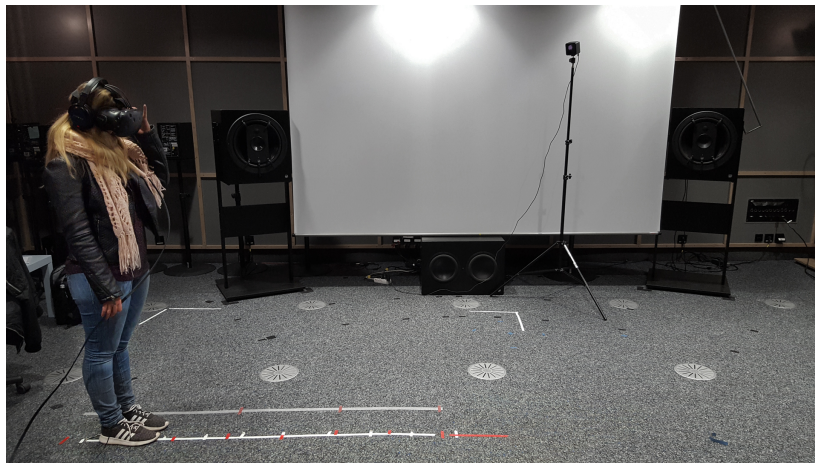
Figure 3.8.: Setup for the dynamic headphone reproduction during the experiment. The participants had to wear an HTC Vive HMD for the tracking and had to walk along the given translation line, which could be seen in the virtual environment as well [237].
