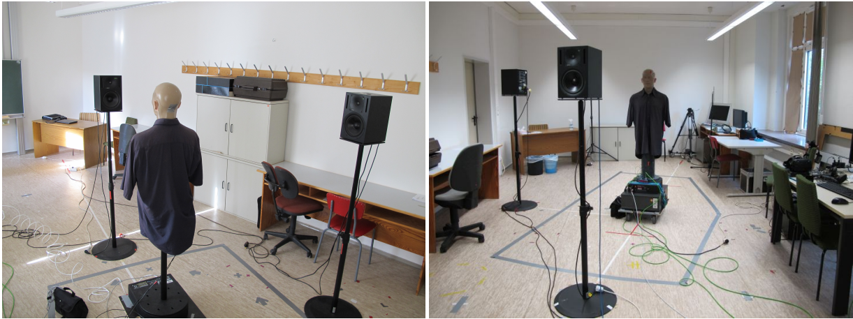
Figure 4.21.: (A) Setup in the seminar room, forming the direct reproduction scenario , where the loudspeakers are turned towards the translation line - (B) Loudspeakers turned by 180° to create an indirect reproduction scenario .
