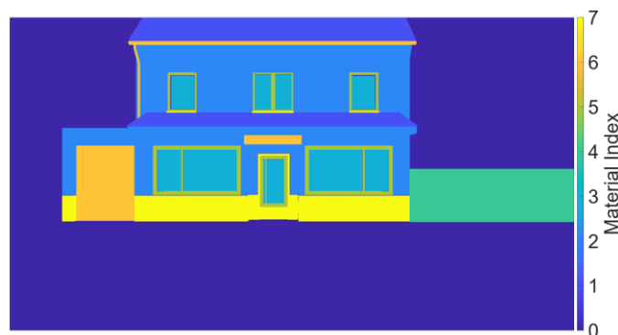
Fig. 3: Material index image. Each recognized material in the scene is assigned a material index from prior knowledge. For the rest, the unknown material index 0 is assigned.
