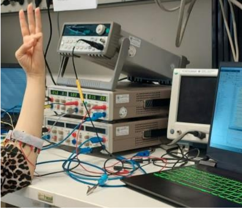
Fig.1: EIT system with 8 electrode band around the forearm of a healthy subject [8]
