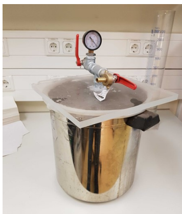
Figure 3. System to generate vacuum and infiltrate several leaves simultaneously.
