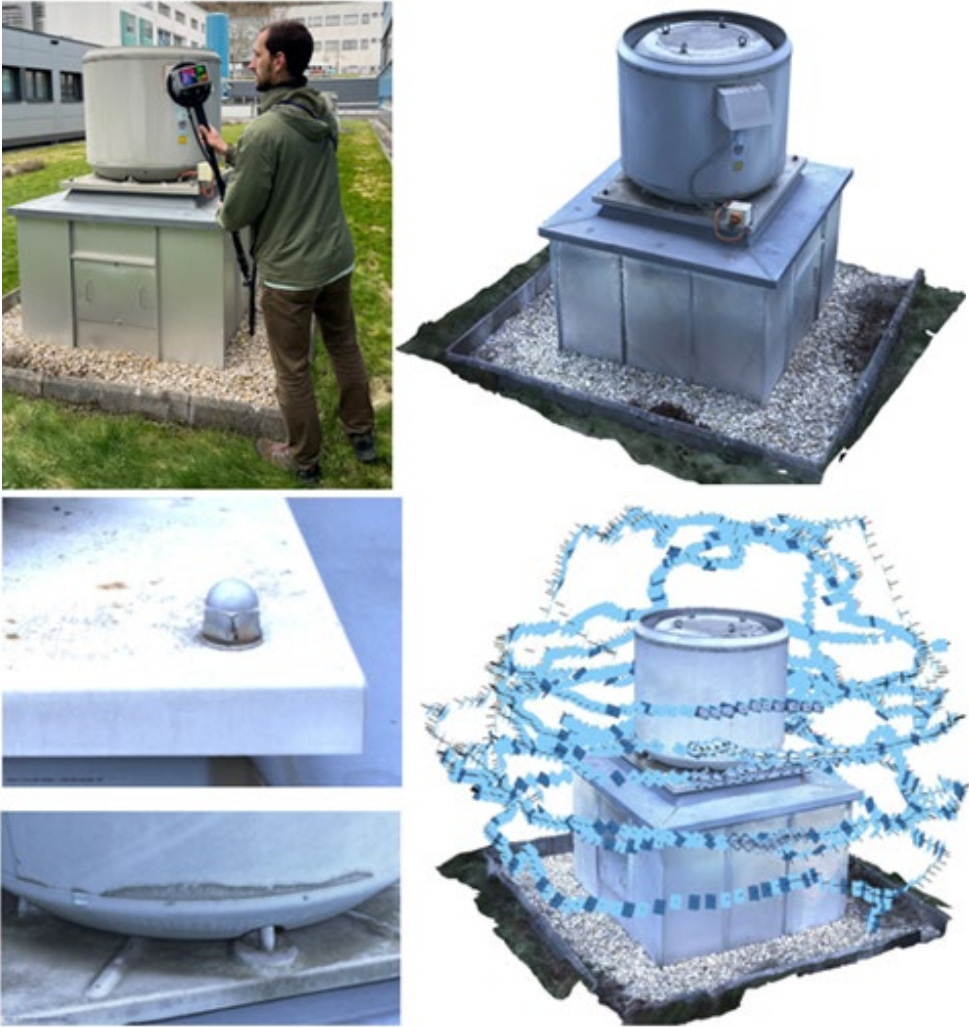
Figure 6: Scanning process (top left), 3D model view (top right), detailed views of potential defects (bottom left), and trajectory of camera positions (bottom right).
