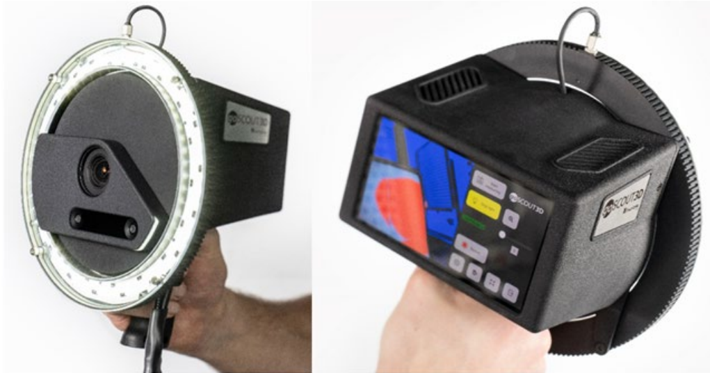
Figure 1: Front and backside of the scanning unit for one-handed operation.
