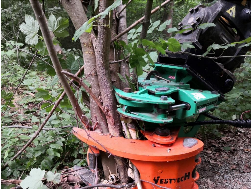
Figure 1: Cutting-and-accumulation unit "Woodcracker C" of the manufacturer "Westtech".
