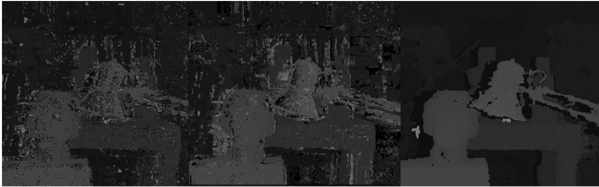
Figure 5 Disparity maps of the Tsukuba pair calculated with the local matcher via CPU (left) local matcher via GPU (middle), and the semi global matcher via CPU with the default 5 search directions(right)
