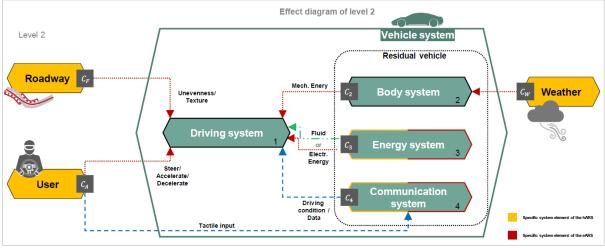
Figure 8: Level 2: Driving System [30]
