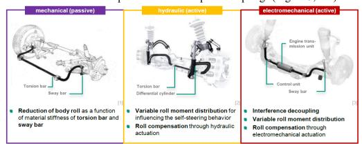
Figure 4: Overview of the alternative reference system elements (RSE) considered for passive, hydraulical active and electromechanical active roll stabilization [30]
