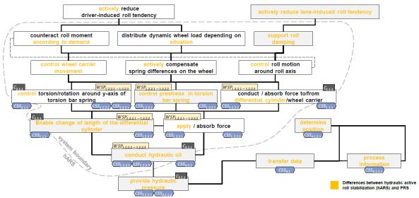
Figure 12: Comparison of the function structure of the hARS and PRS [30]
