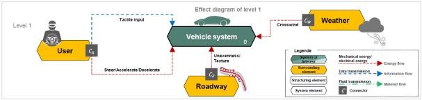
Figure 7: Level 1: Vehicle System [30]
