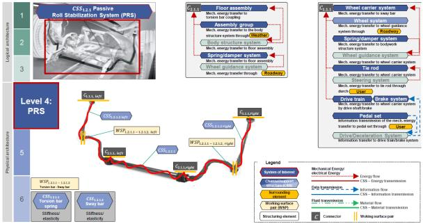
Figure 10: C&C<sup>2</sup> model on level 4: Passive Roll Stabilization (PRS) [30]
