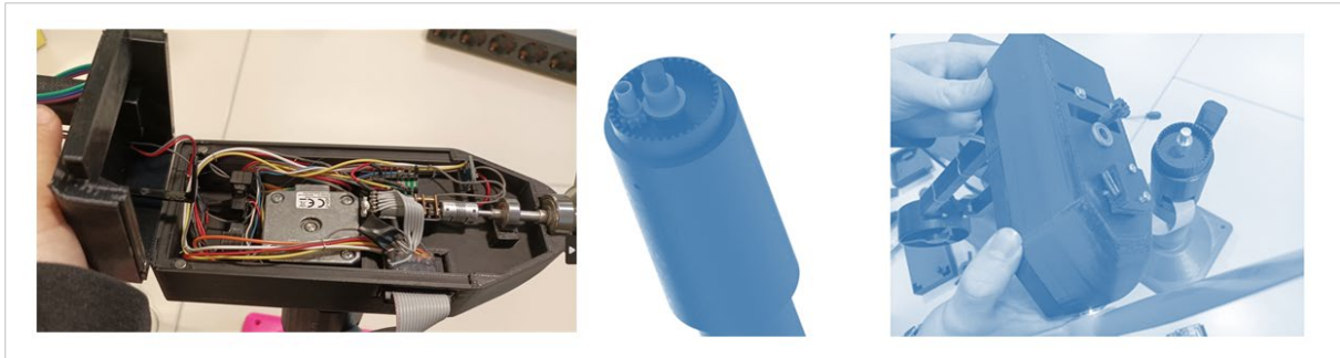
Figure 5: Insight into the redesigned gondola (left), CAD-view (middle), underside gondola with limit switches (right)
