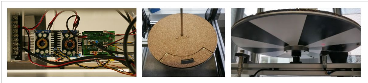
Figure 12: Electrical components (left picture), top and bottom of the rotary disc (middle and right picture),
