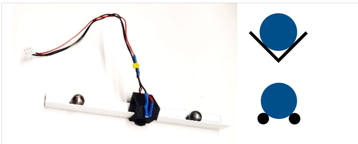
Figure 10: Developed solution for the horizontal ball transport
