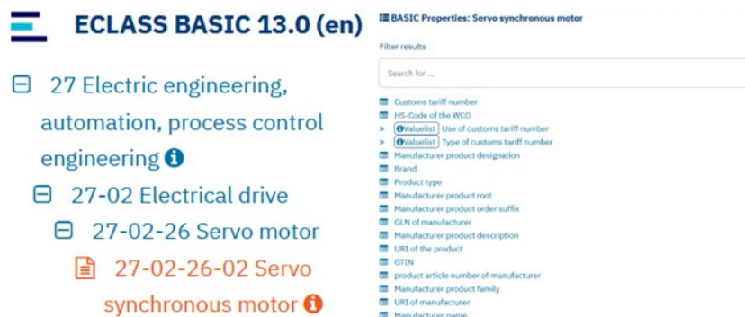
Figure 4: Product properties – ECLASS entry “27-02-26-02 Servo synchronous motor” [7]
