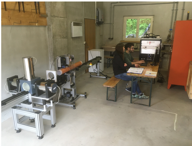
Figure 3. Field lab near the drill site containing the MSCL scanner (photo by Sebastian Schaller).
