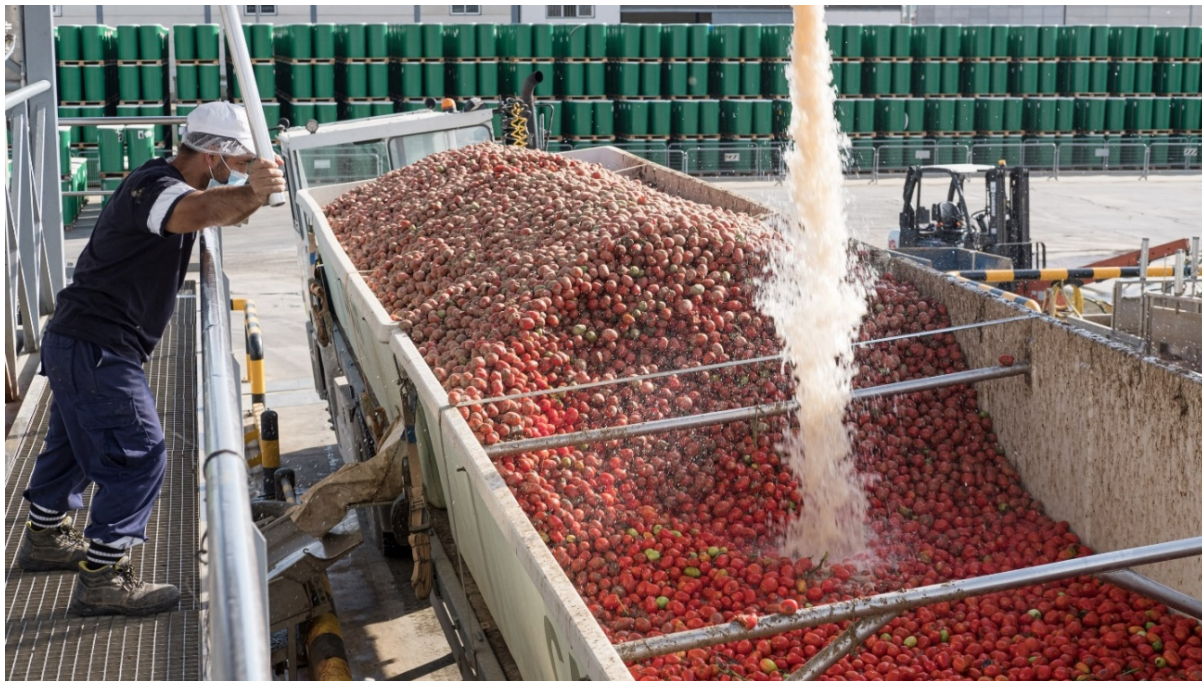
Figure 8. Tomatoes being washed and pushed into the conveyor system.
