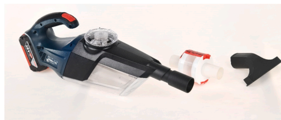
Fig. 1. Bosch GAS18V-1 vacuum cleaner and Sirchie 6197E filter unit used for Total Human DNA Sampling.
