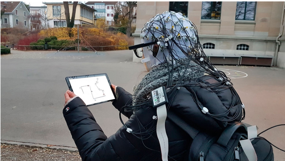
Figure 3. Real-time ambulatory assessment of a navigator's visual attention using mobile eye tracking (mET) and mobile encephalography (mEEG) measurements to assess cognitive load in during a mGID assisted wayfinding task outdoors (Fabrikant, 2022: Fig. 5).
