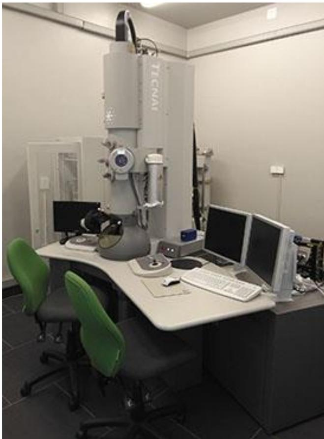
Figure 2.1: FEI TECNAI T20 TEM used in this thesis.
