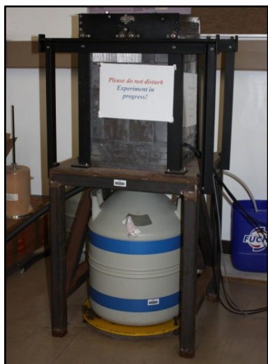
Figure 47: The HPGe Detector: Model GC4530
