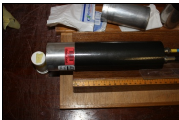
Figure 46: The Thin-Window NaI Detector Coupled to a PMT
