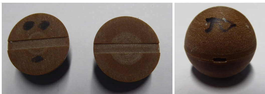
Figure 55: Solid Water Eye Phantom for TLD Measurements in the “Claws”
