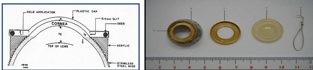
Figure 17: Applicator Designed to Irradiate Blood Vessels Growing into the Cornea
