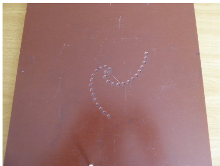
Figure 52: Solid Water Phantom with Slots for TLD Radial Dose Function Measurements
