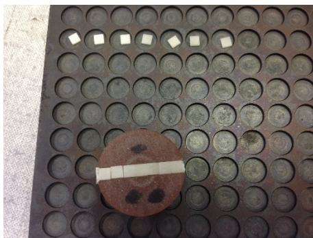
Figure 57: Seven TLDs in the Phantom
