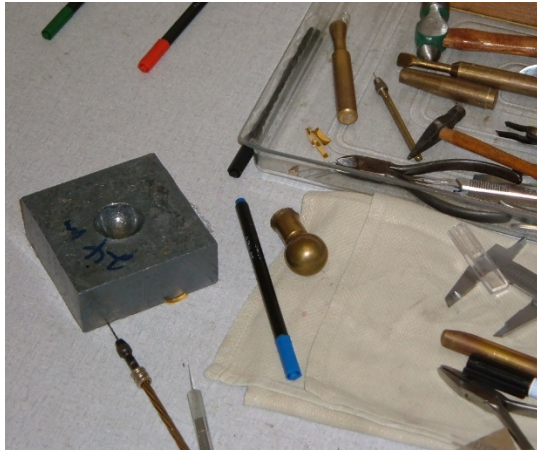
Figure 3: The Flat Gold Plate is Shaped in a Lead Mould to the Correct Curvature
