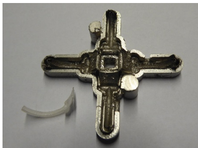
Figure 66: The Woods Metal Insert Used for Stabilization During the Manufacture of the Legs
