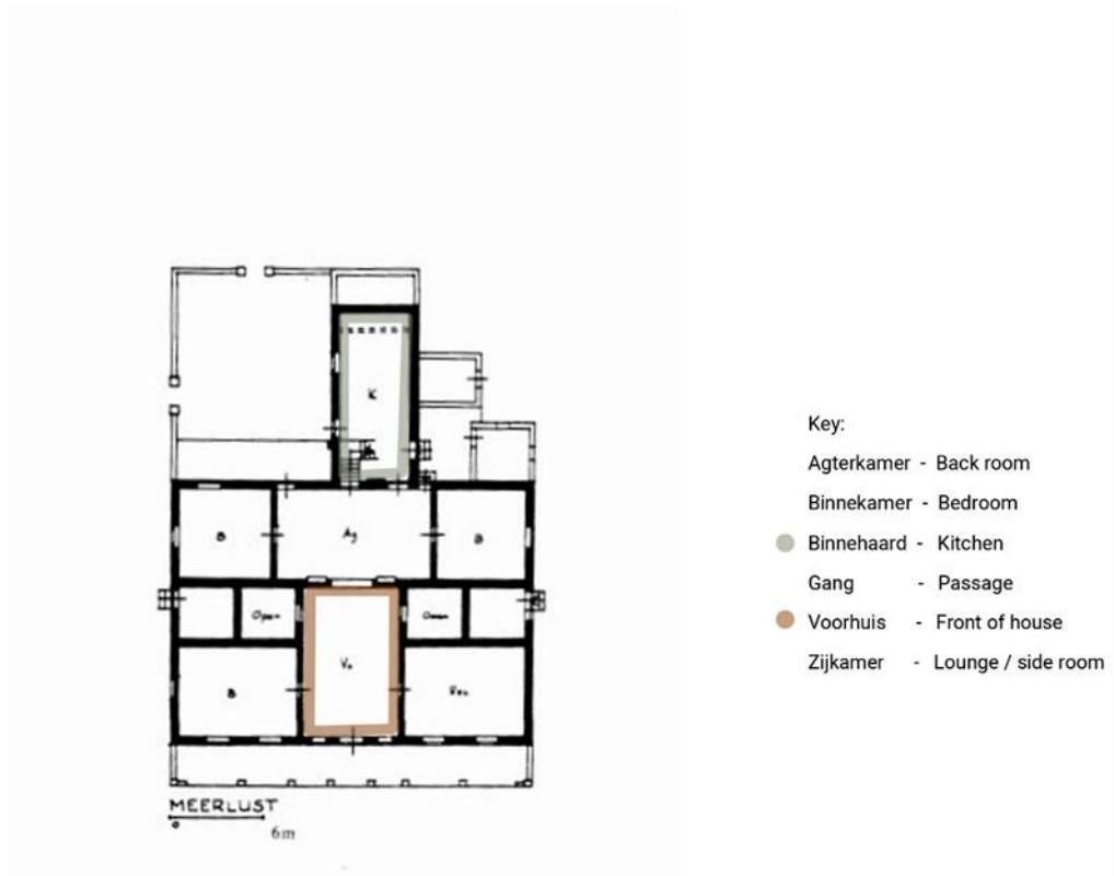
Figure 6: Floor plan of Meerlust showing the relation of the voorhuis and the kitchen
