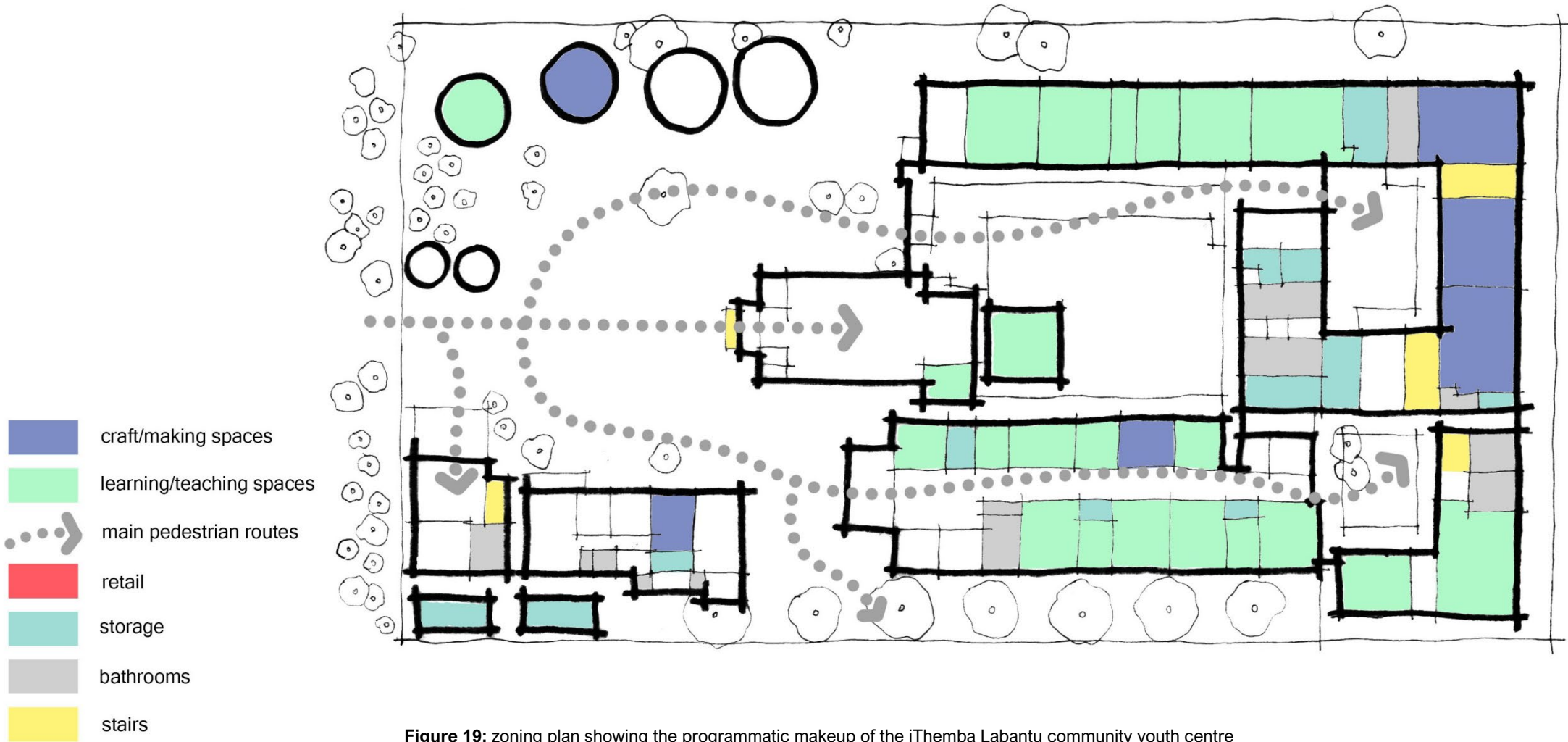
Figure 19: zoning plan showing the programmatic makeup of the iThemba Labantu community youth centre
