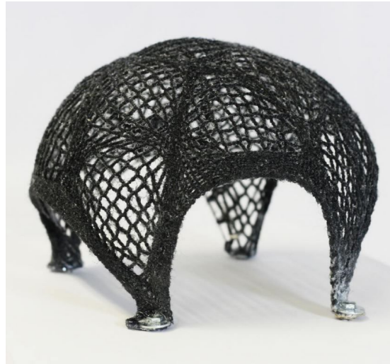
Figure 62: a knit sample cast in resin to hold a rigid shape
