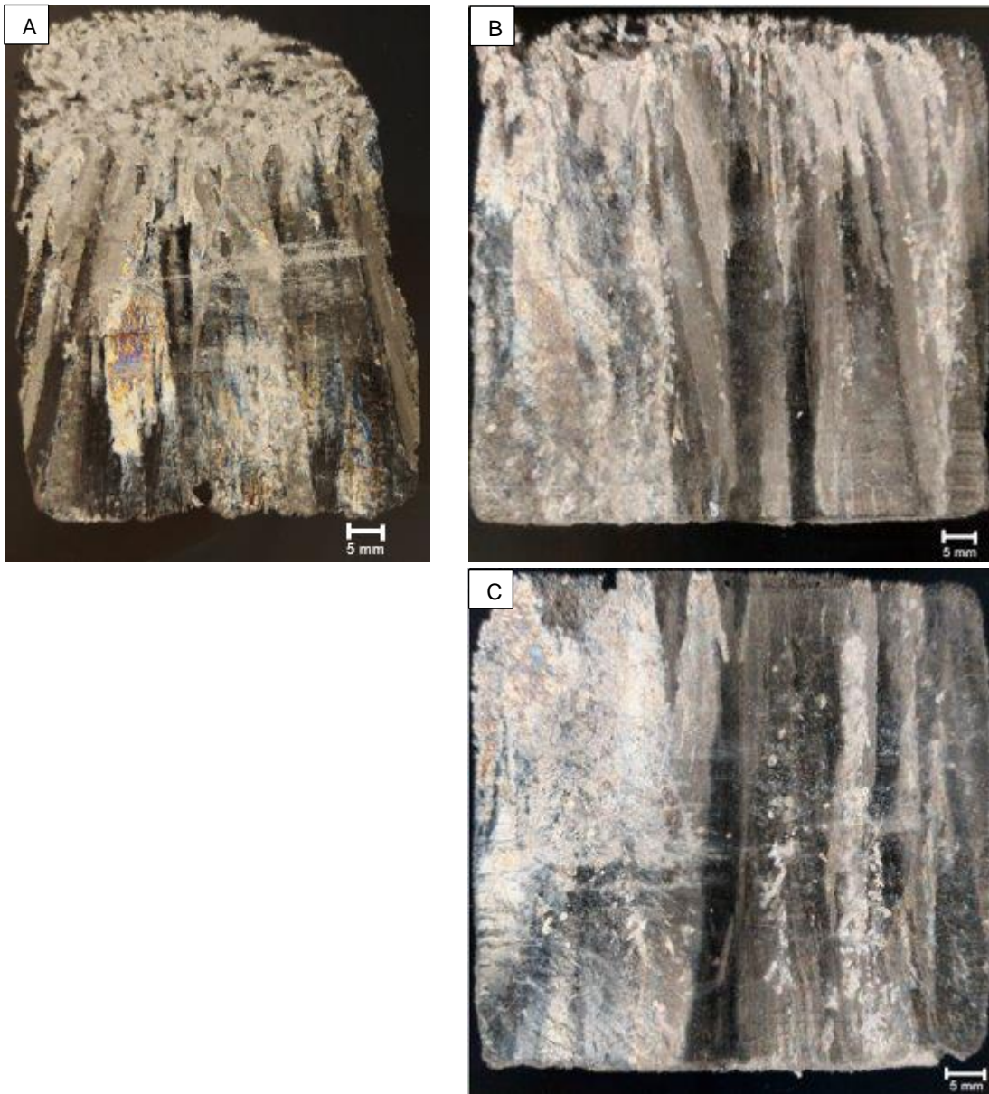
Figure E. 3 Cross polarisation results of samples grown at -20°C from solutions of starting artificial ocean salinity of 30 psu from a (A) 3 L and (B) 30 L reactor.
