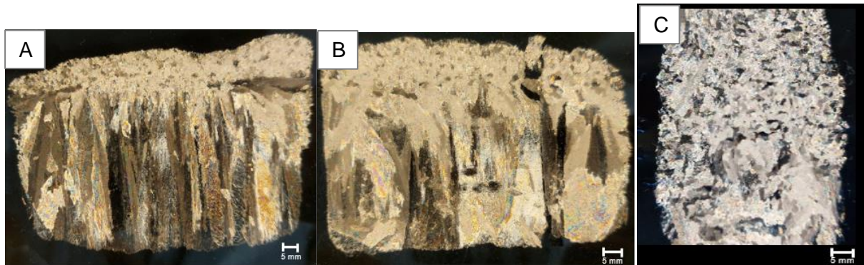
Figure 5-1 Visual results of ice grown at -20°C from a 10 psu solution at (A) 0 rpm, (B) 800 rpm and (C) 1800 rpm stirring speed.
