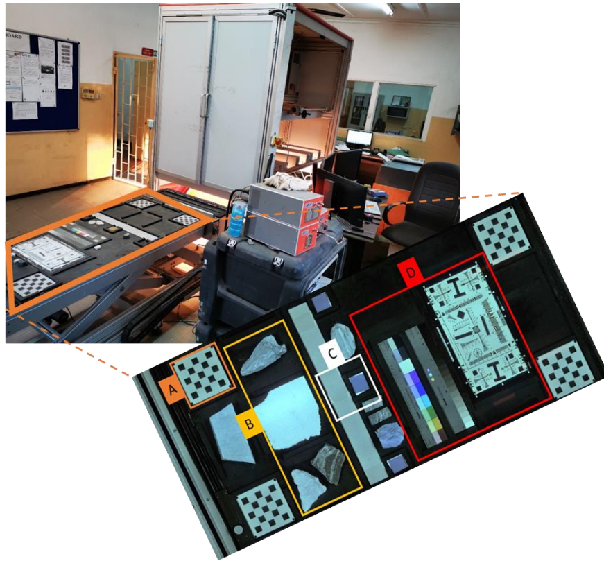
Figure 3.3: Calibration board for the HSI system calibration. The calibration board is placed under the system cameras, moving in the conveyor belt. A: anodized aluminium squares are used to ensure image completeness and correct aspect ratio. B: examples of standard materials used to ensure spectral calibration, the centre object being a slab of styrofoam. C: reference glass and plastic are used to ensure camera calibration. D: Kodak colour and focus sheets to ensure correct colour balance, focus, and aspect ratio (Photo courtesy of Terracore).
