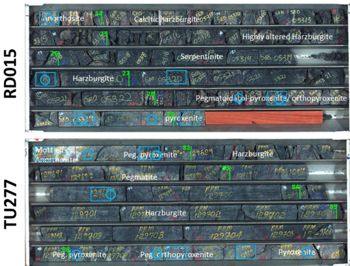
Figure 4.1: Photographs of TU277 and RD015 drill cores investigated with the selected marked areas for QEMSCAN (circles) and QXRD (rectangle) analyses sampled on the drill cores. Core depths are indicated with green lines marking the change in lithologies with associated changes in mineral assemblage and texture. TU277 core depths are labelled from 82 m to 86 m and RD015 from 25 m to 29 m.
