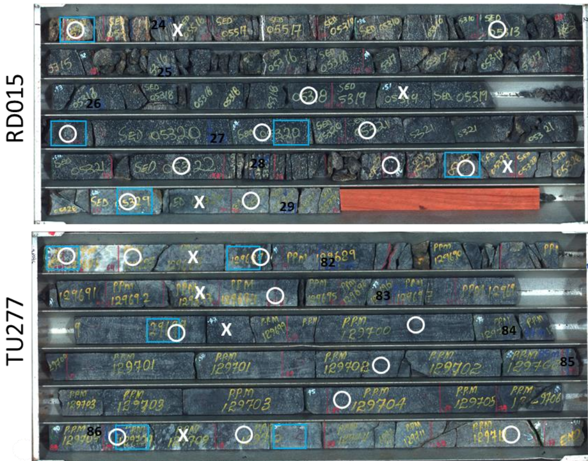
Figure 3.2: Selected areas for mini core extraction (circles), XQRD samples (blue rectangles), and rescanned HSI core (marked with X).
