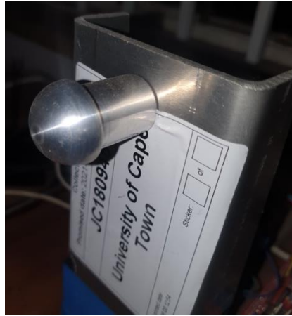
Figure 60: 25mm indenter installed into system.
