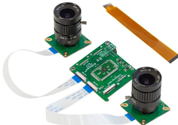
Figure 34: Arducam 12MP Synchronized Stereo Camera.
