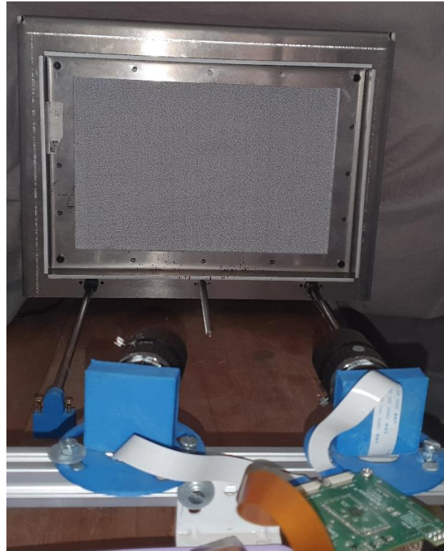
Figure 52: Displacement Measurement Equipment Setup
