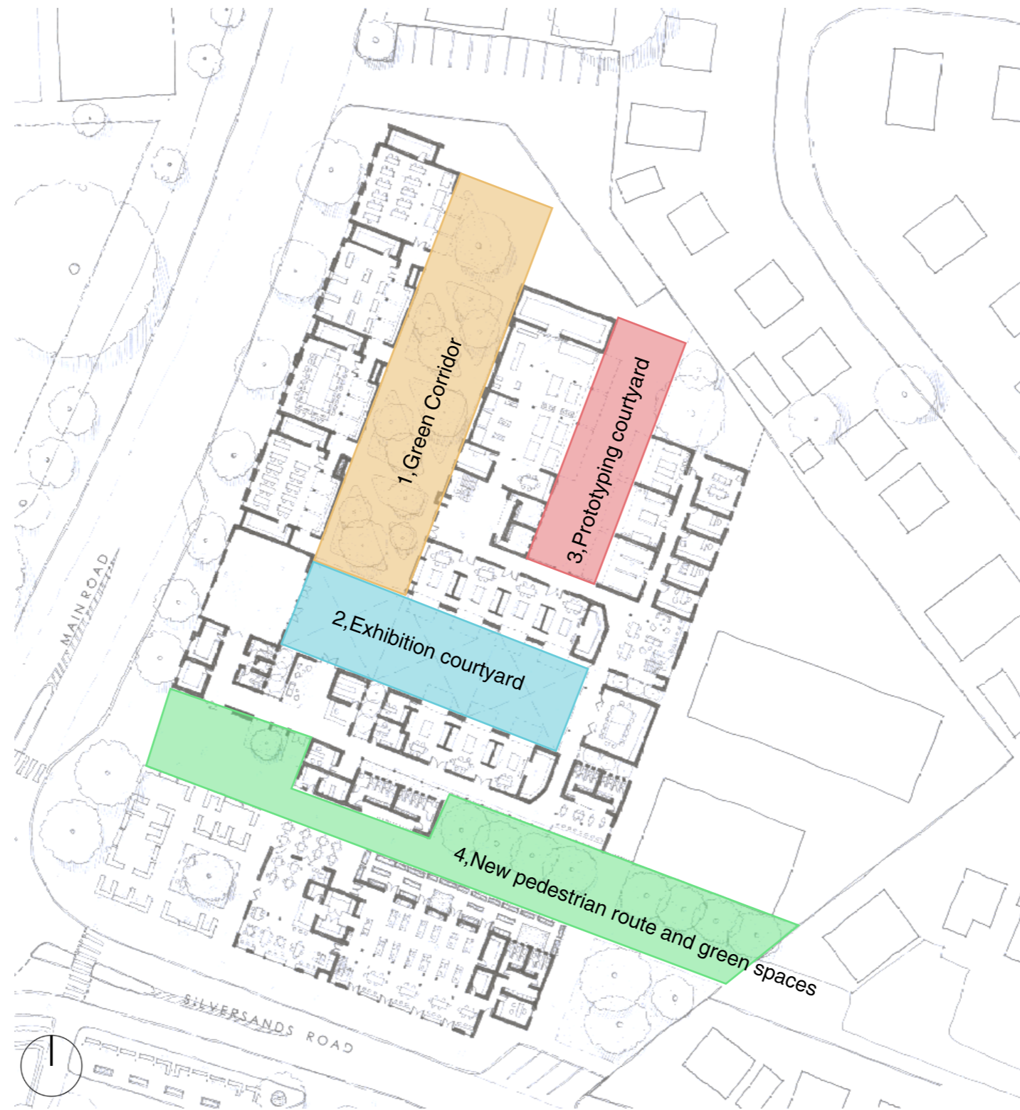
Figure 85 Courtyard development of the Skills Centre (by the author, 2022)
