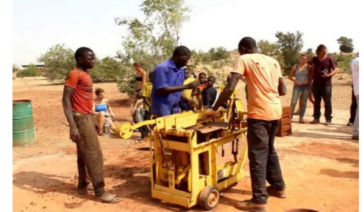
Figure 7 Production of earth bricks being pressed on size (How to produce a brick with clay and community. 2014)
