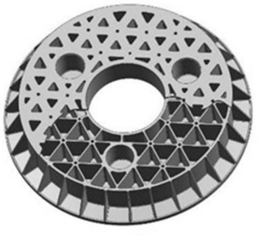
Figure 2.8 Primary Mirror design for 760 mm diameter.
